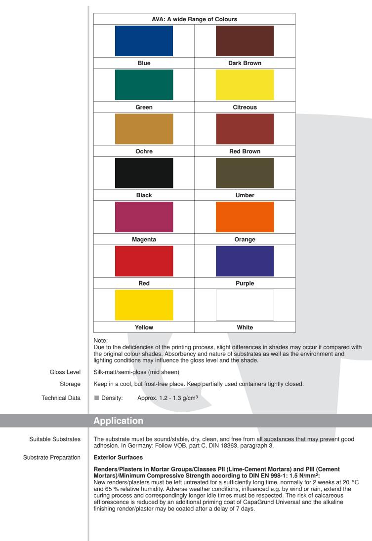
Existing renders/plasters: Repairs must have adequate time to cure and dry. Highly porous, absorbent, slightly sanding renders/plasters: Apply one priming coat of OptiGrund E.L.F. Prime highly sanding, chalking renders/plasters with Dupa-grund. Coat mineral lightweight renders/plasters of mortar group PII with Sylitol or AmphiSilan products.
